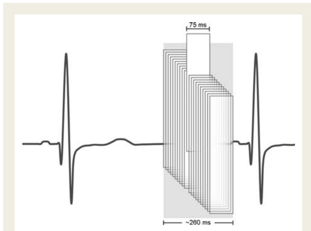
Figure 1 Image reconstruction in prospectively ECG-triggered high-pitch spiral coronary CT angiography using dual-source CT. The entire period of data acquisition is approximately 260 ms long and is placed in diastole. Images are reconstructed using a half-scan reconstruction algorithm. The temporal resolution of each cross-sectional image is 75 ms. While the first (most cranial) image is reconstructed at the beginning of the 260 ms data window, subsequent images are reconstructed slightly later in the cardiac cycle.
